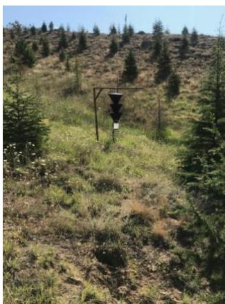
Figure 1. Scandinavian type pheromone trap with three funnels.
