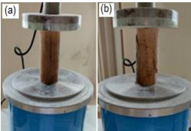
Figure 5. Sample before unconfined compressive test (a) and after test (b)
