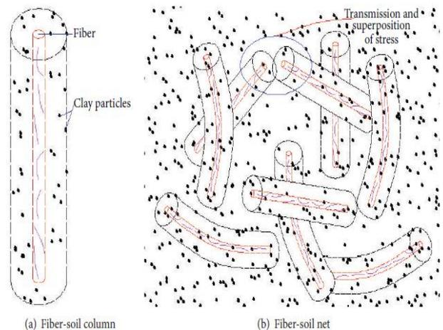
Figure 1. Model of fiber and soil column – net [3]
