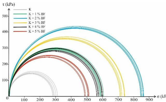
**Figure 8.** Mohr graphs of unreinforced clay and BF reinforced samples
