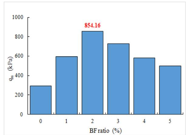
**Figure 9.** The relation of  $q_u$  - BF ratio of unreinforced and reinforced clay samples
