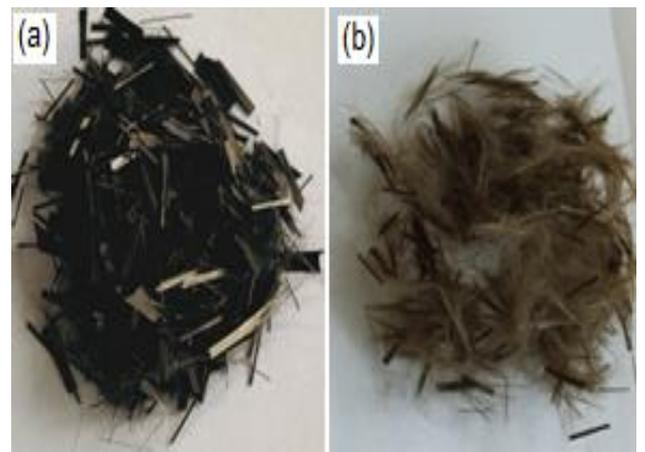
Figure 3. Unseparated (a) and separated (b) BF used in the study
