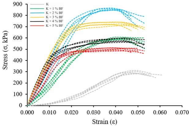
**Figure 7.** Stress – strain curves of unreinforced K and BF reinforced samples
