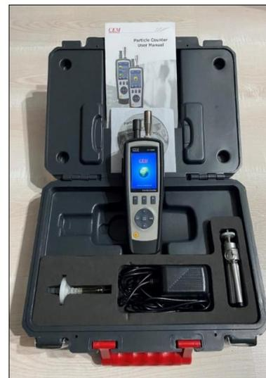
Figure 4. PM<sub>10</sub> measurement device
