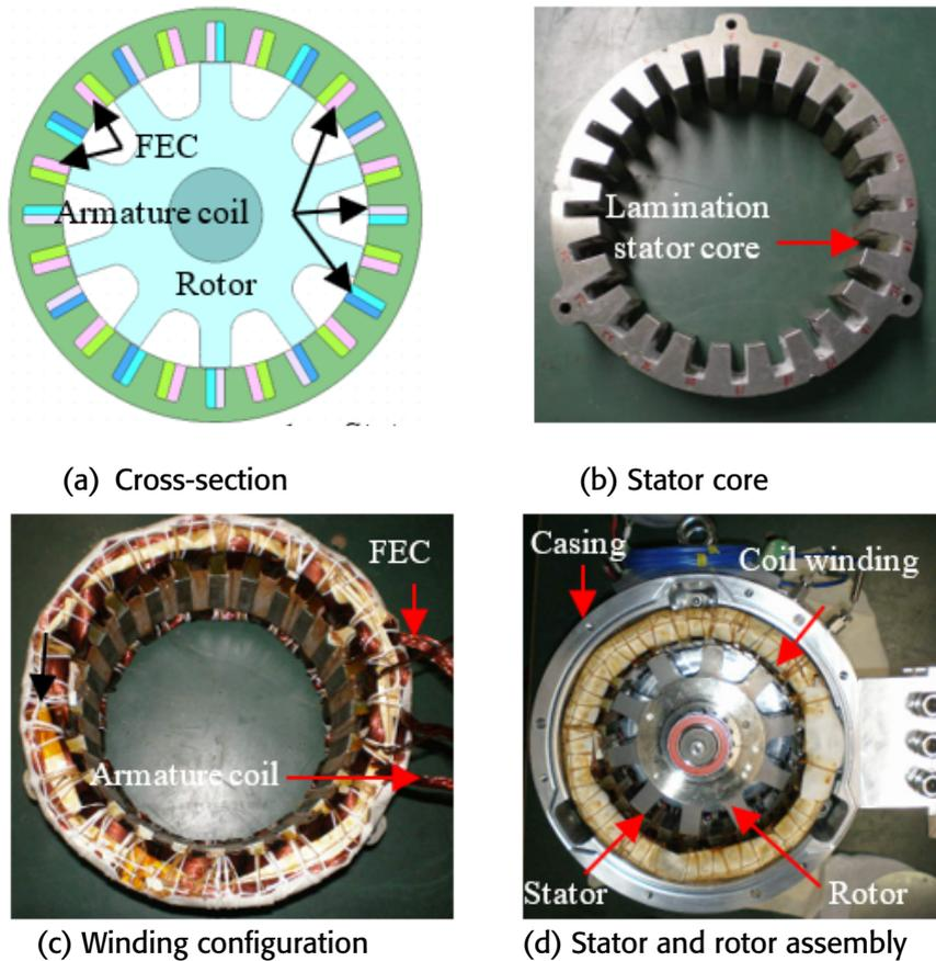
Figure 5. 24S-10 configuration of salient rotor FEFSM [56]
