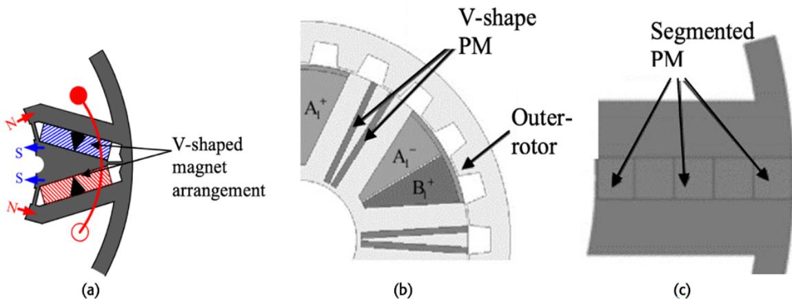
Figure 11. Magnet-V-shaped (a) rotor inner, (b) rotor-outer, (c) magnet-segmented
