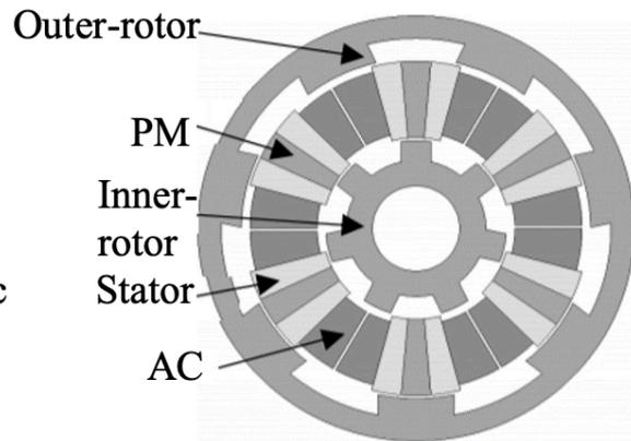
Figure 3. Dual rotor structure PMFSM.
