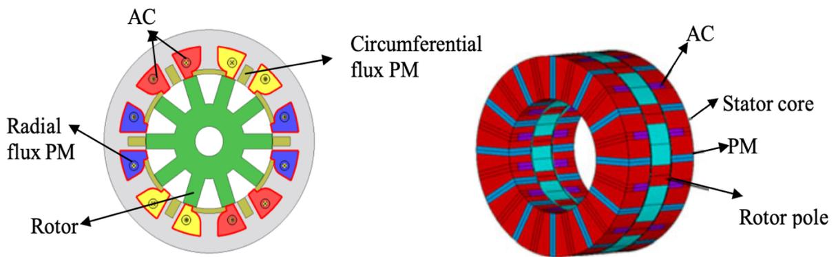
Figure 10. (a) Circumferential arrangement of the magnet (b) Double stator axial flux machine
