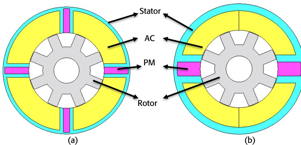
Figure 1. Configuration of PMFSM (a) 4S/8P (b) 2S/8P
