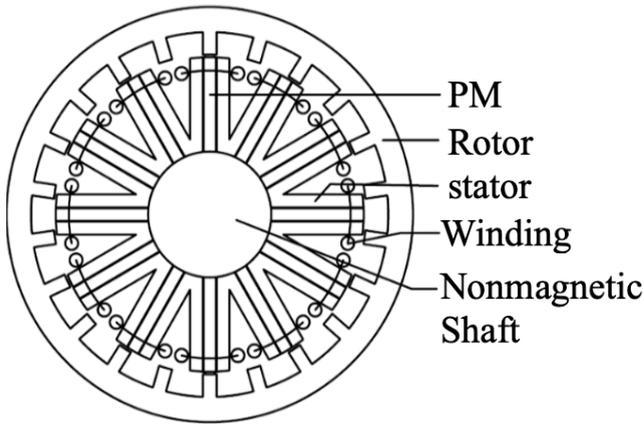
Figure 2. Outer-rotor PMFSM
