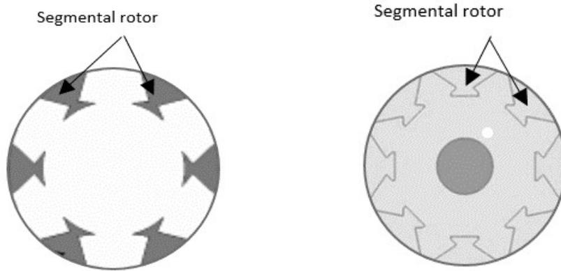
Figure 9. Segmental rotor (a) 6-rotor pole (b) 8-rotor pole
