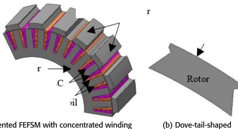
Figure 7. Odd rotor pole, three-phase outer rotor 36S-21P (a) non-overlap windings FEFSM, (b) Dove-tail-shaped [64]
