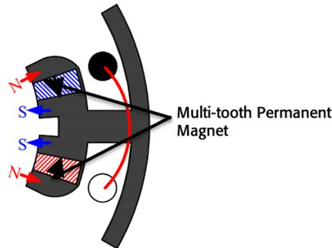
Figure 12. Cross-sectional view of multi-toothed machine
