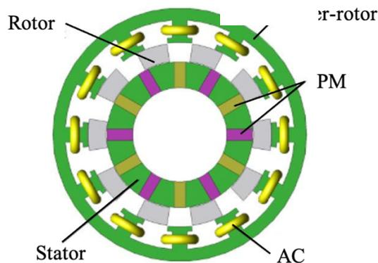
Figure 4. Dual-stator structure of PMFSM
