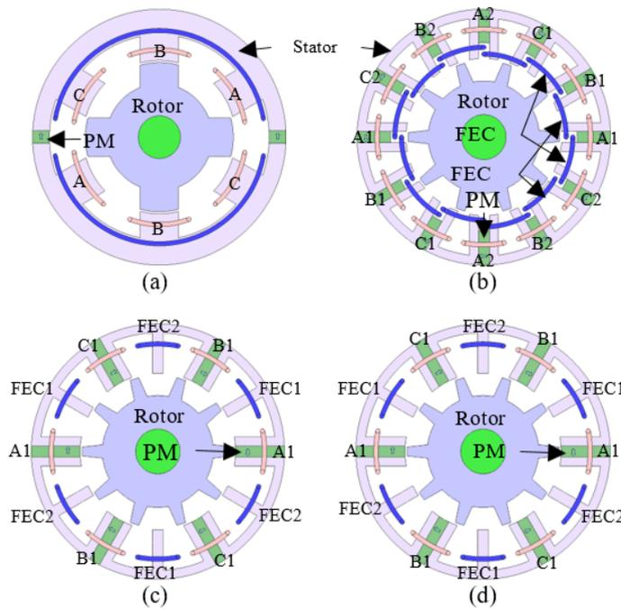
Fig. 8. HEFSM three-phase, (a) 6S 4P, (b) C-core 12S-10P, (c) E core 12S-10P, and (d) E-core 6S-8P E core [65-69].
