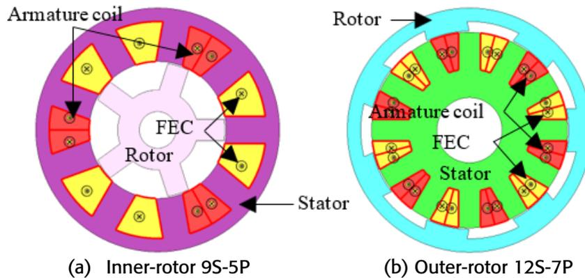
Figure 6. Three-phase, overlap windings with odd rotor poles FEFSM [56].
