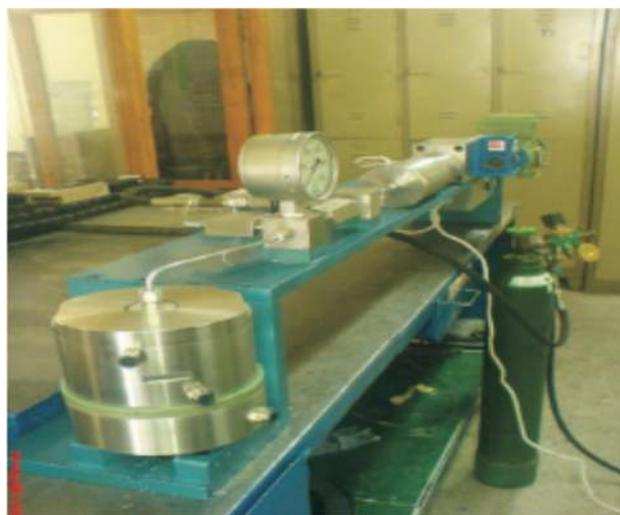
Fig 1. High Pressure Differential Thermal Analysis Device
