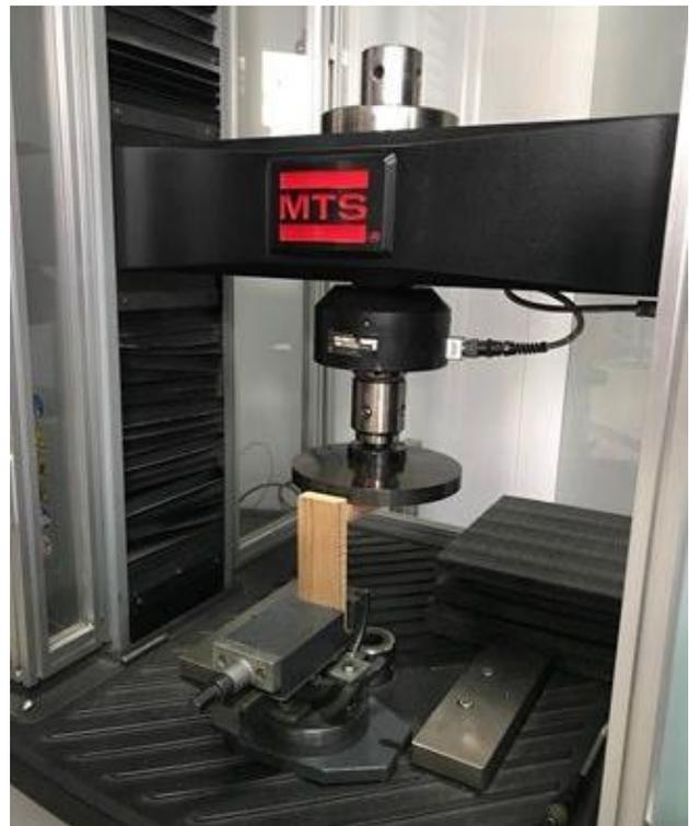
Figure 3. MTS Universal testing machine
