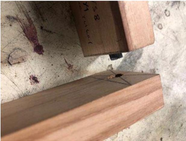
Figure 8. Plastic Dowel Failure
