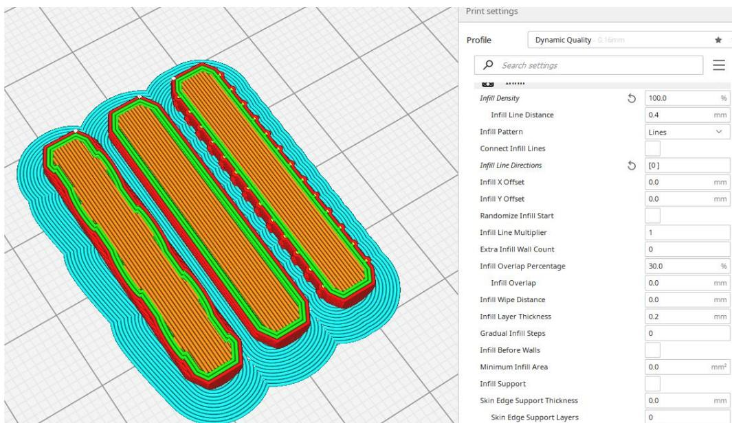
Figure 1. Infill line directions of 3 D printed dowels
