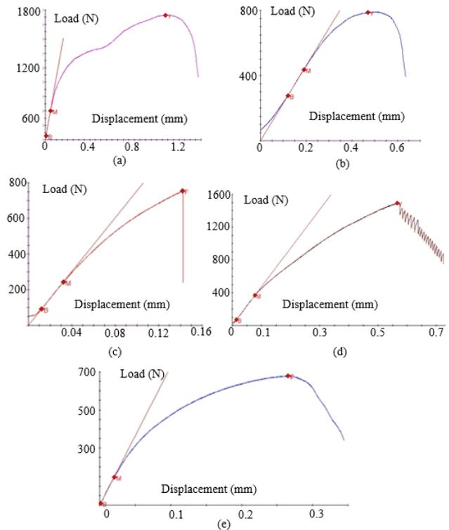
Figure 9. Typical load-displacement curve for L-joint a) with only PLA dowel, b) with PLA + TPU dowels, c) with resin dowel, d) with commercially available wood dowels e) with commercially available plastic dowel.
