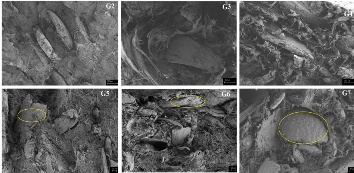
**Figure 6.** SEM images of samples (G2: 10% branch flour added sample, G3: 20% branch flour added sample, G4: 40% branch flour added sample, G5: 10% leaf flour added sample, G6: 20% leaf flour added sample, G7: 40% leaf flour added sample)
