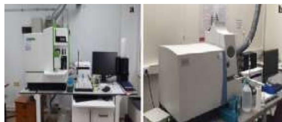
Figure 4. Measurement of ICP analyse (a-ICP-OES, b-ICP-MS)
