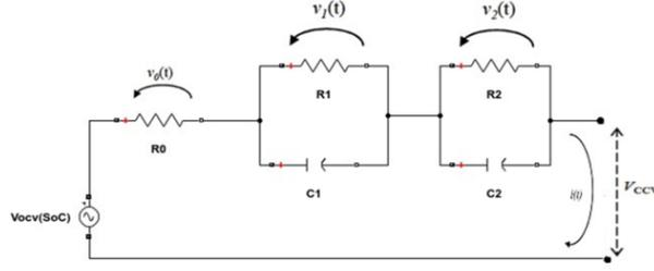
**Figure 1.** Second order Randles electrical equivalent circuit
