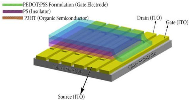
Figure 1. OFET's ITO/PS/PEDOT:PSS based schematic structure.
