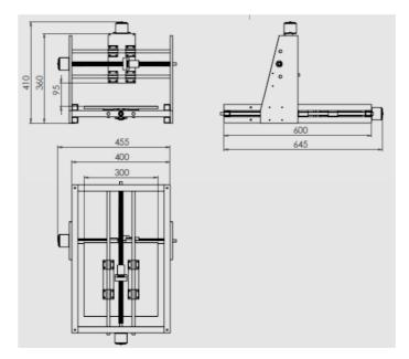
Figure 5. Technical Drawing Measurements of a Three-Axis Mini CNC Machine
