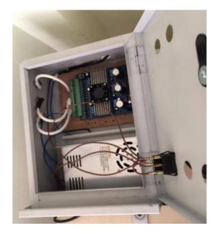
Figure 9. Driver Card and Power Supply Panel
