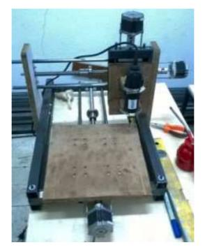
Figure 4. Fully Assembled View of a Three-Axis Mini CNC Machine
