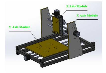
Figure 3. Solid Model of a three-axis Mini CNC Machine
