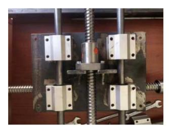
Figure 8. Ball Screw Nut
