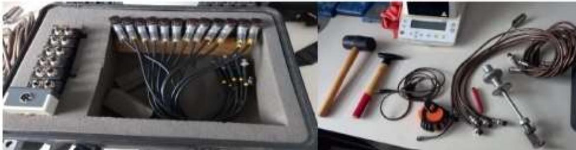
Figure 1. Acoustic tomography equipment
