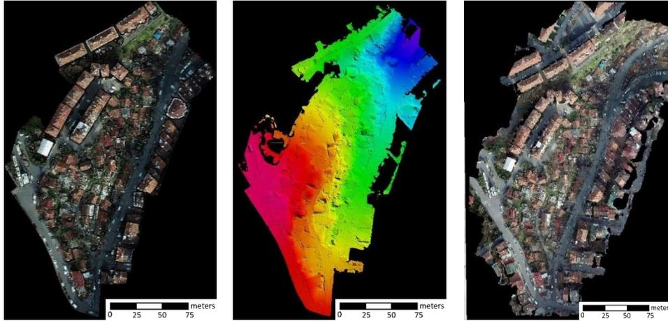
Fig. 3. Colored Dense Point Cloud, Digital Elevation Model (DEM) and Orthomosaic.
