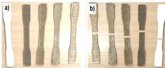
Fig. 3. Tensile performance polypropylene composite samples a) before test and b) after test
