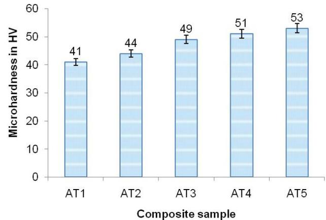
Fig. 4. Microhardness behaviour of polypropylene composites
