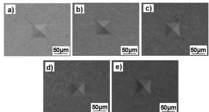
Fig. 5. Optical microscope image of microhardness tested samples a) AT1, b) AT2, c) AT3, d) AT4, and e) AT5
