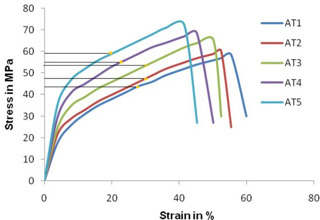
Fig. 2. Stress-strain curve for polypropylene composites
