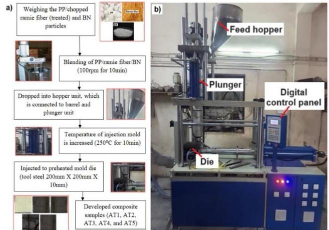
Fig. 1. a) Flow process chart for composite fabrication and b) Injection moulding setup
