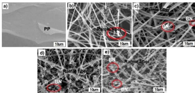
Fig. 6. SEM analysis of polypropylene composites a) AT1, b) AT2, c) AT3, d) AT4, and e) AT5
