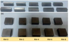
Fig. 1. Produced by hot pressing process: (a) Three-point bending test samples, (b) Friction-wear test samples
