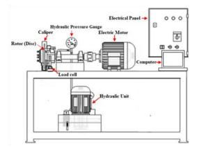
Fig. 3. Friction wear tester [48]
