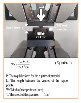
Fig. 2. TRS test set up
