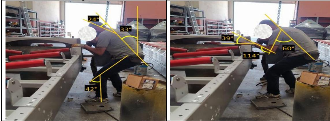
During the assembly of the drum, roller, and electric motor, the belt chassis is placed on a support from both sides. There is a high risk of workplace accidents if any falling incident occurs during the operation.
