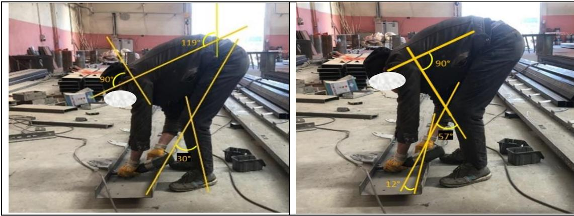
In the third stage, the connection of the main chassis is completed. The A (5) and B (2) scores for the two main chassis, joined by bolts and nuts, were matched in the C table, resulting in a score of 4 (Table 10). With the addition of the activity score, the REBA score was determined to be 5. The risk level for this task falls within the range of 4-7, indicating a medium risk level. As per the REBA guidelines, precautions should be taken to mitigate the risks associated with this posture.
