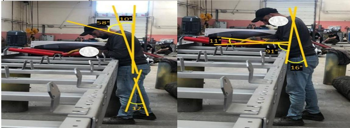
In the final stage of the assembly, the electric motor is mounted (Table 14). Upon examining Table 14, the A score was found to be 8, and the B score was 7. When the A and B scores were matched in the C table, the score was determined to be 10. With the addition of the activity score, the REBA score for the electric motor assembly was calculated as 13. This score corresponds to a degree of 4, indicating a very high-risk level, and according to the REBA guidelines, immediate action must be taken.
