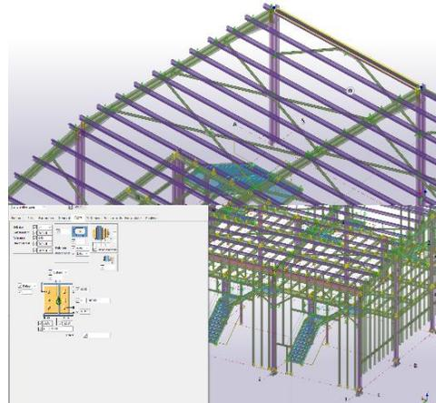
**Figure 7.** Purlin & Diagonal Structural Elements and Facade Tiling & Anchor Modeling.
