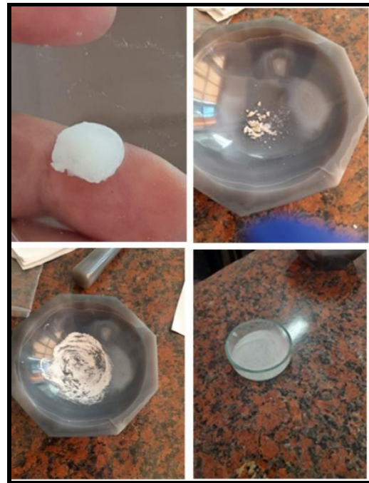
Figure 5. Powder Preparation from otoliths with agate mortar and drying after treatment H 2 O 2
