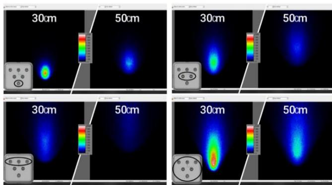
Figure 6. Visible color and light intensity on the dark concrete surface at heights of 30 cm (left) and 50 cm (right) obtained in ANSYS Speos software.
