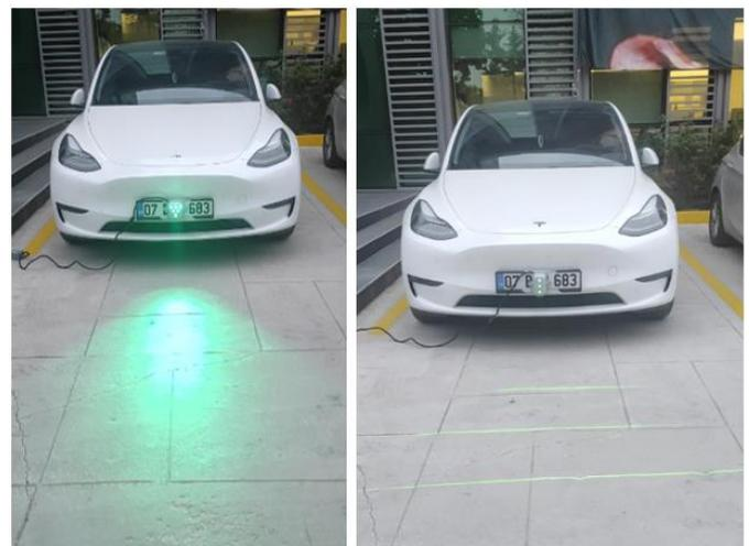
Figure 11. 50 cm Height- OVAS System with LED and Lazer Light Source
