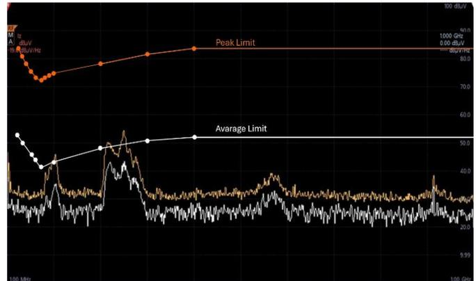
Figure 7. Emission Measurement with Near Field Probe.
