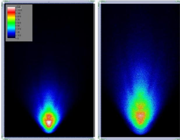
Figure 9. Diagram of Isolux Values from the Center Analyzed at 30 cm and 50 cm Heights.
