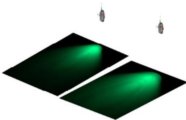
Figure 5. Lux value map of LED-based OVAS formed on the ground at 30 cm and 50 cm heights obtained in ANSYS Speos software.
