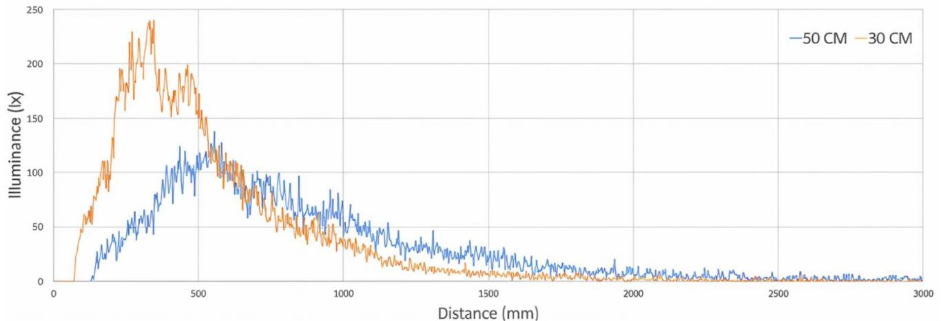
Figure 12. Illuminance (lx) variation as a function of distance (mm) for the OVAS system using LED light source at 30 cm and 50 cm heights on the vehicle front.
