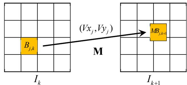
Figure 1. Motion estimation (ME) between video frames.
