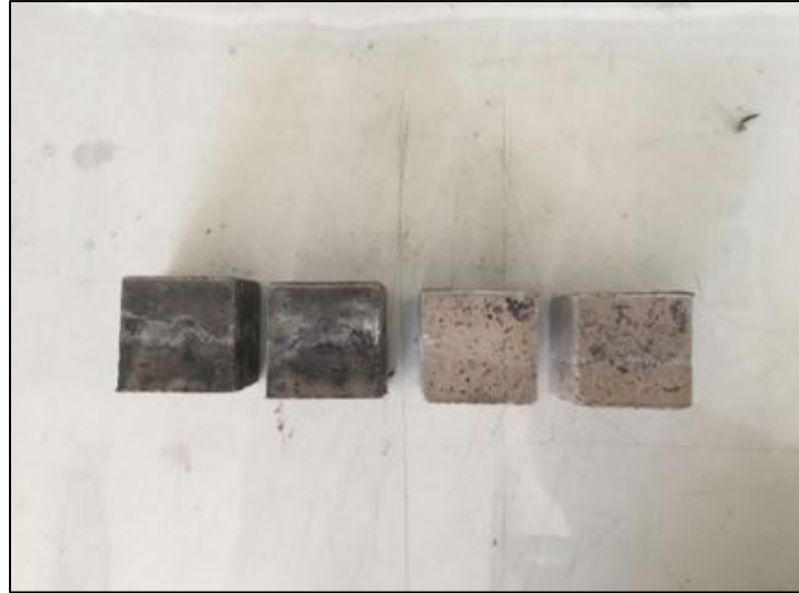
Figure 7. Post-high-temperature views of the blends (from left to right: O-0, O-30, T-0, and T-30)
