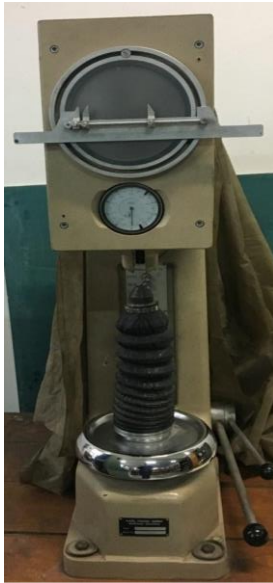
Figure 2. Karl Frank Universal Hardness Tester.
