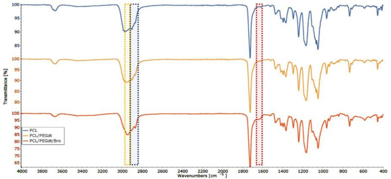
**Figure 2.** FTIR Spectra of PCL (blue line), PCL/PEGdt (yellow line; [PCL]: 10% (w:v) and [PEGdt]: 2.5% (w:v) and PCL/PEGdt/Bro (orange line; [PCL]: 10% (w:v), [PEGdt]: 2.5% (w:v), and [Bro]: 0.25% (w:v)). Each component's specific regions are highlighted with dotted boxes that match the colors of the lines.
