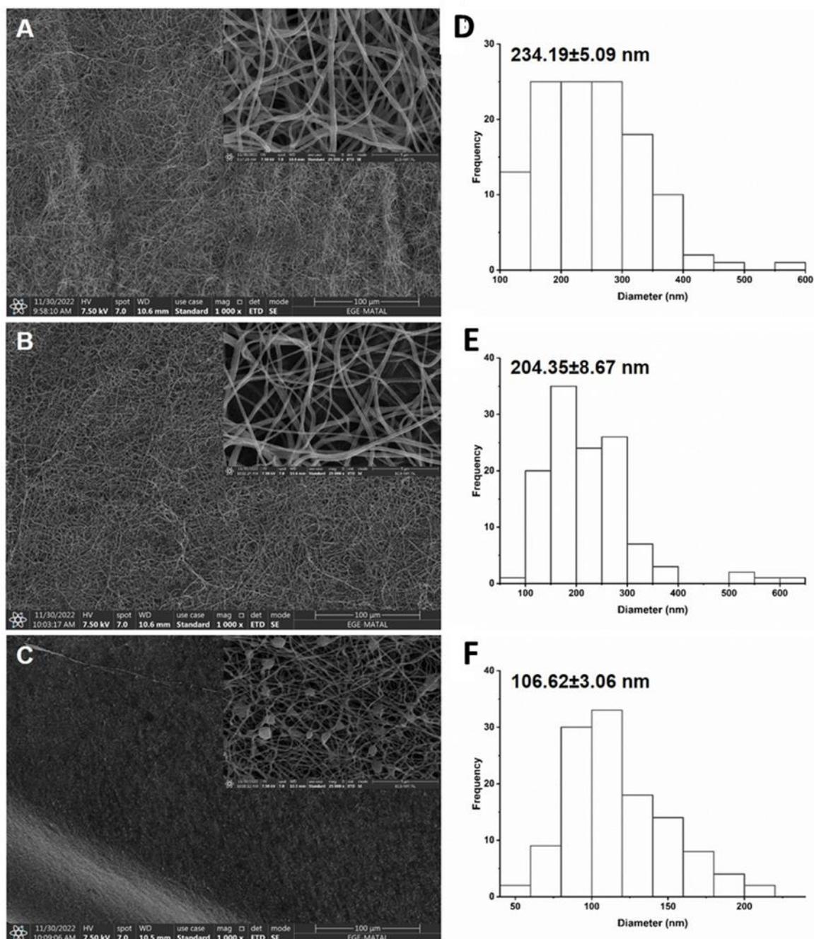
**Figure 1.** SEM micrographs of **A)** PCL (10%; w:v), **B)** PCL/PEGdt ([PCL]: 10%; w:v and [PEGdt]: 2.5%; w:v), **C)** PCL/PEGdt ENs ([PCL]: 10%; w:v and [PEGdt]: 5.0%; w:v) (Magnification 1000X, scale bar 100 µm and for inset figures, magnification 25000X, scale bar 5 µm). Histogram for ENs diameter distribution and average diameters of **D)** PCL (10%; w:v), **E)** PCL/PEGdt ([PCL]: 10%; w:v and [PEGdt]: 2.5%; w:v), **F)** PCL/PEGdt ENs ([PCL]: 10%; w:v and [PEGdt]: 5.0%; w:v).
