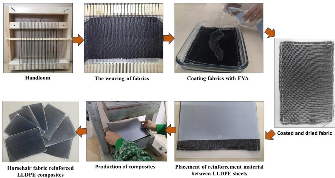
**Figure 1.** The production stages of composite samples
