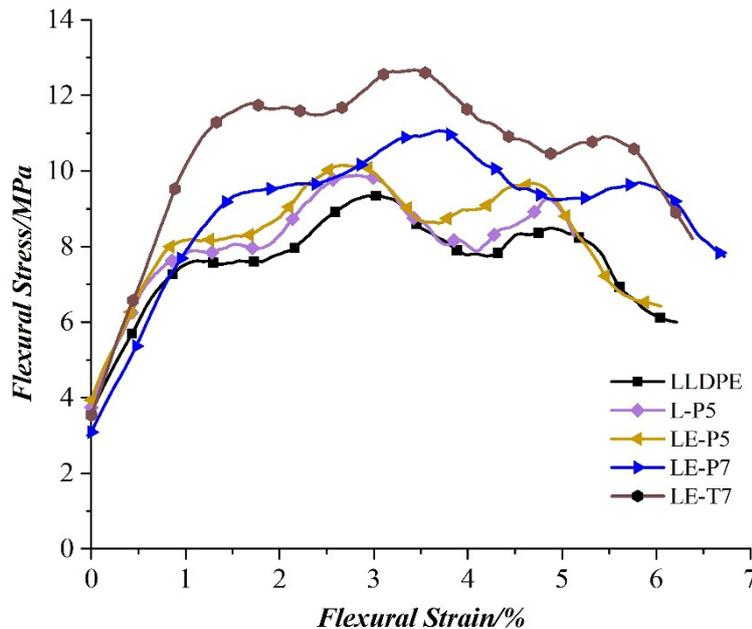
Figure 6. Flexural stress-strain curves of composite samples in the weft direction
