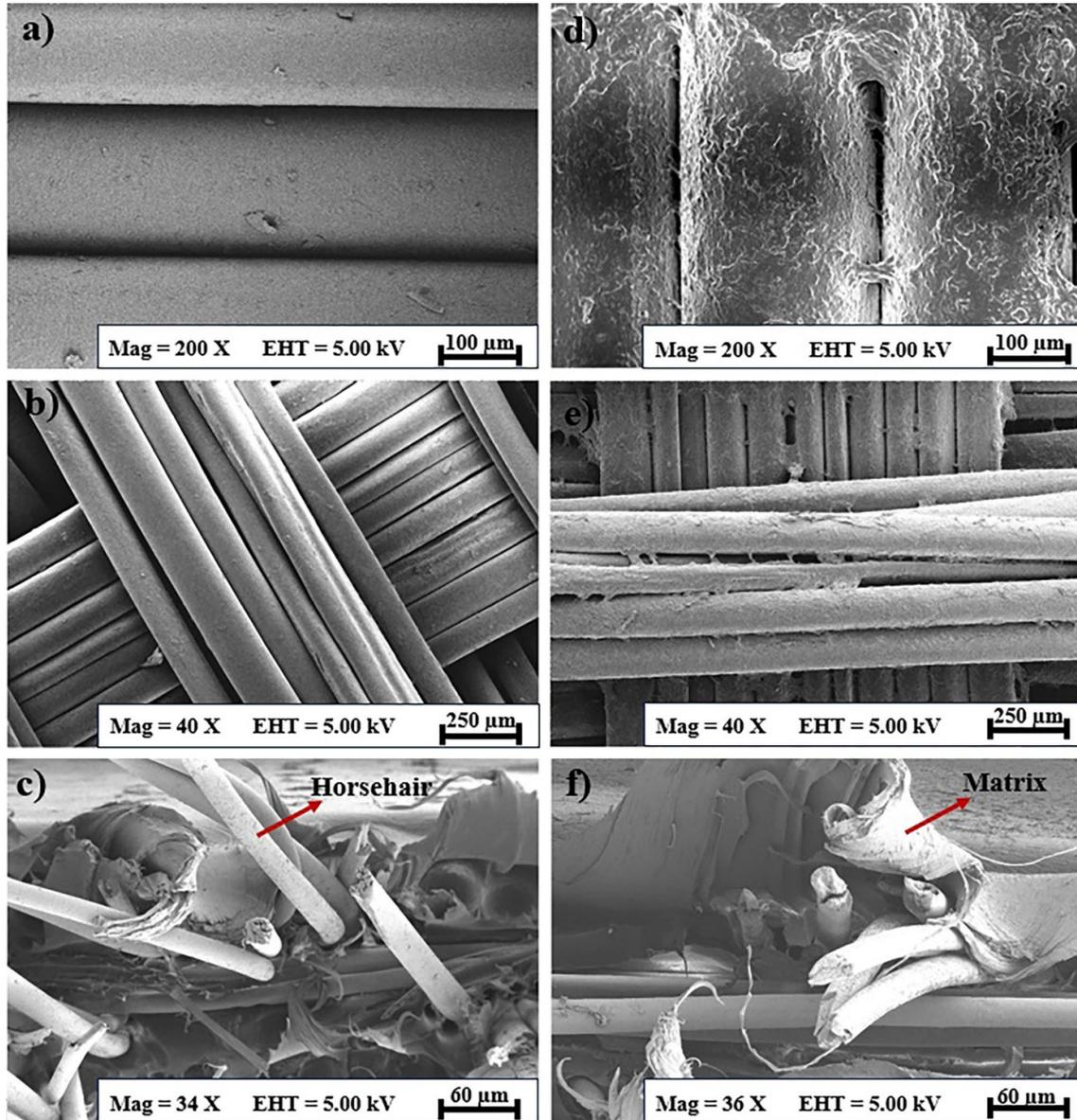
**Figure 5.** FE-SEM micrographs of untreated (a, b) and EVA-treated (d, e) fabrics at 200X and 40X magnifications; micrographs of tensile fracture surfaces of composites in the weft direction (c) L-P5 at 34X and (f) LE-P5 composites at 36X
