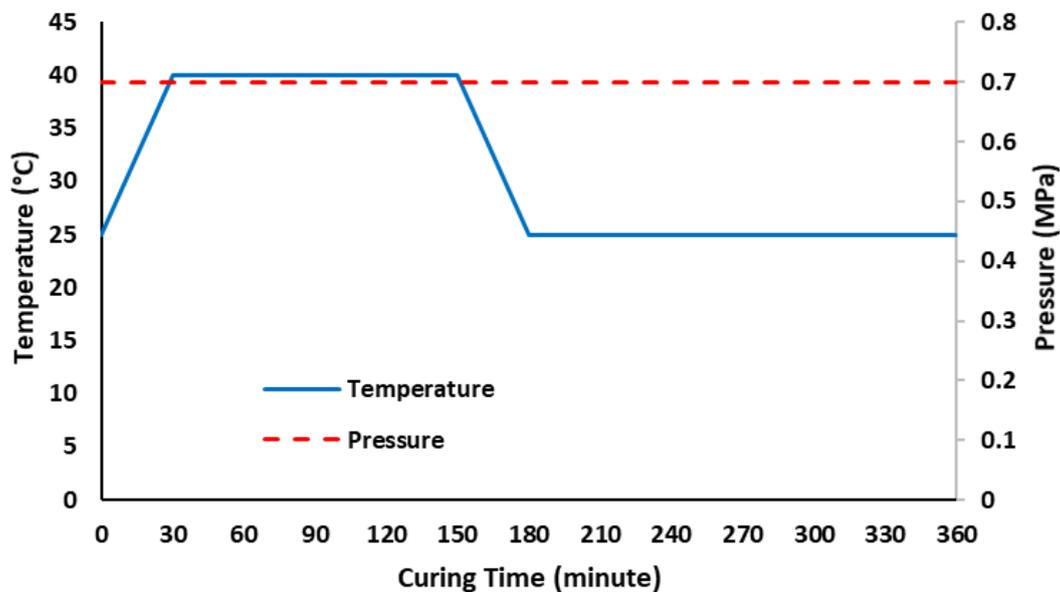
**Figure 1.** Composite plate production condition
