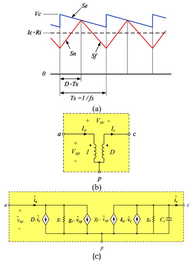
Figure 2. Pwm-switch model with peak current-mode control in CCM (a) Significant control signal waveforms (b) dc equivalent circuit (c) ac equivalent circuit.
