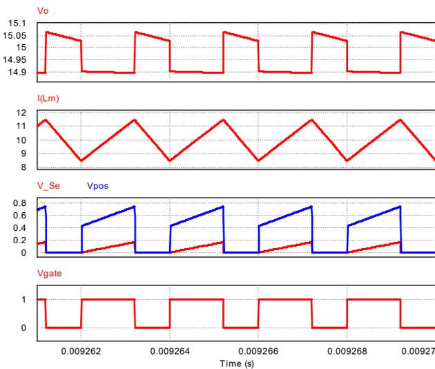
Figure 7. PSIM time domain simulation waveforms of the flyback converter in Fig. 6.
