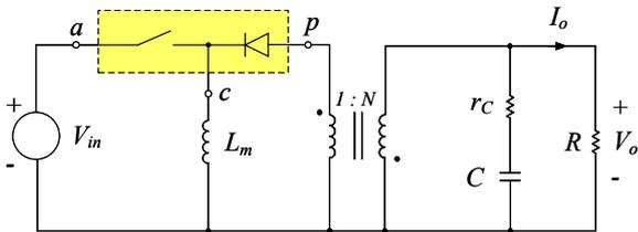
Figure 3. Representation of flyback converter by the pwm-switch model
