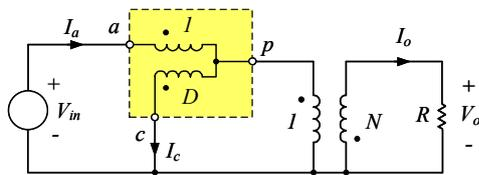
Figure 4. Dc pwm-switch equivalent circuit of flyback converter in Fig. 3.
