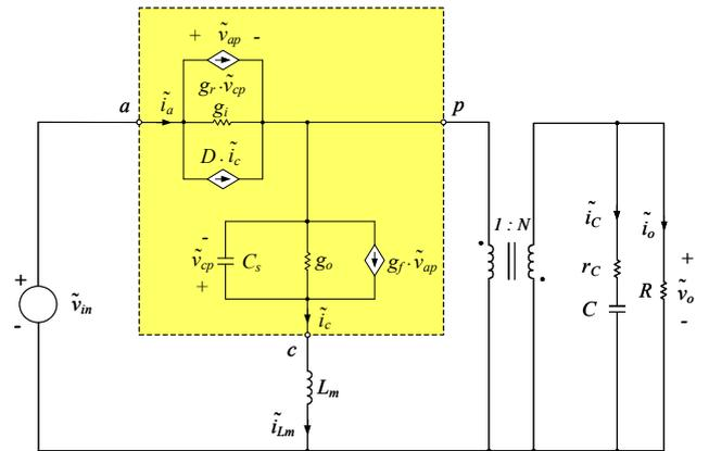
Figure 5. Ac small signal pwm-switch model of flyback converter.
