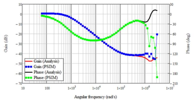
Figure 8. Bode plot comparisons of the example flyback converter as simulated by PSIM and calculated by (10).
