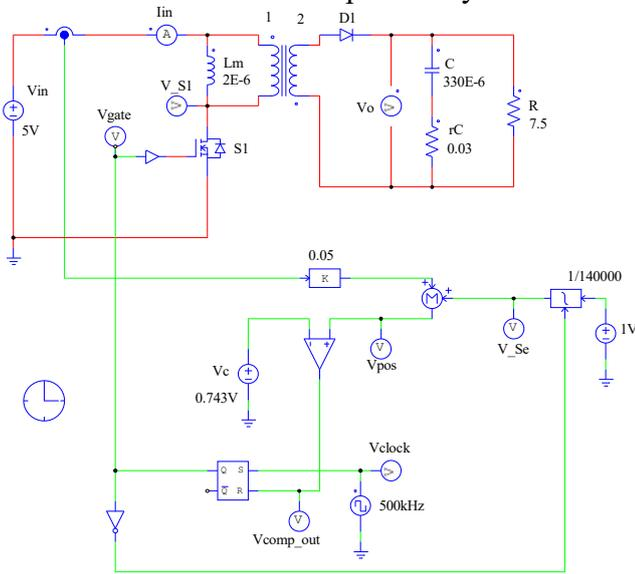
Figure 6. Switching model of the flyback converter for time domain PSIM simulations.
