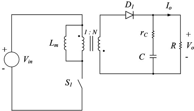
Figure 1. Circuit diagram of flyback converter.
