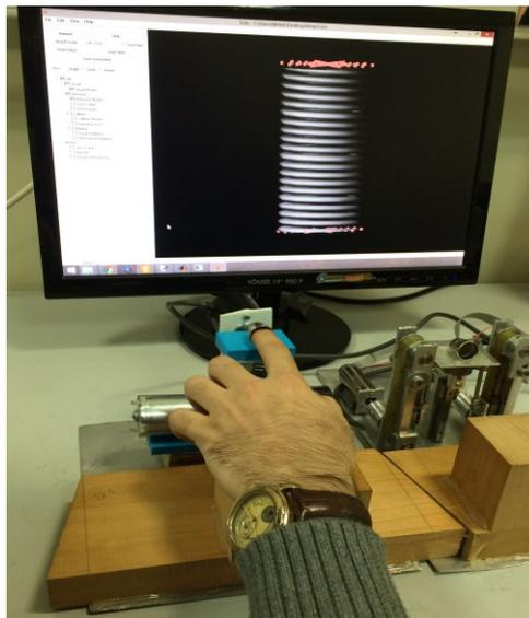
**Figure 1.** Experimental setup consists of a 2-DOF haptic interface, a 2-DOF input device, a 6-DOF force sensor, two vibration motors, and a virtual environment
