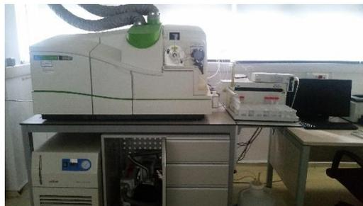
Figure 3. Nexion 300D model ICP-MS
