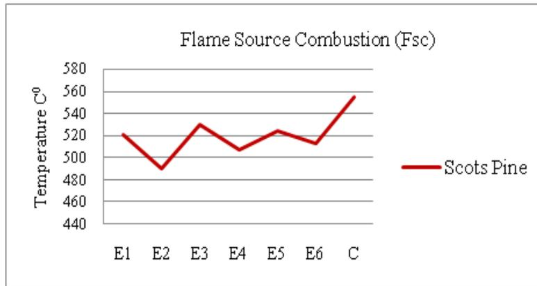
**Figure 2.** Fsc temperature values of Scots pine test samples according to impregnation compositions
