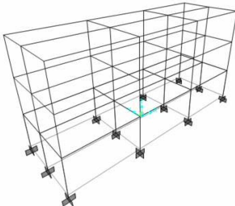
Figure 5: 3 Storey 3 Dimensional Frame (SAP2000)
