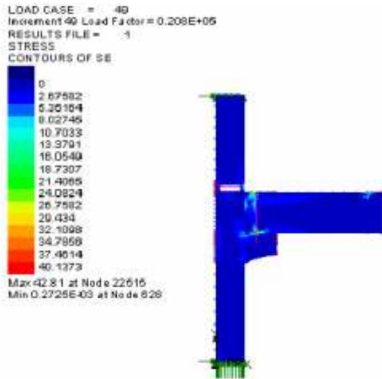
Figure 13: Von Mises Stress for Corbel +Plate + Stiffener Model
