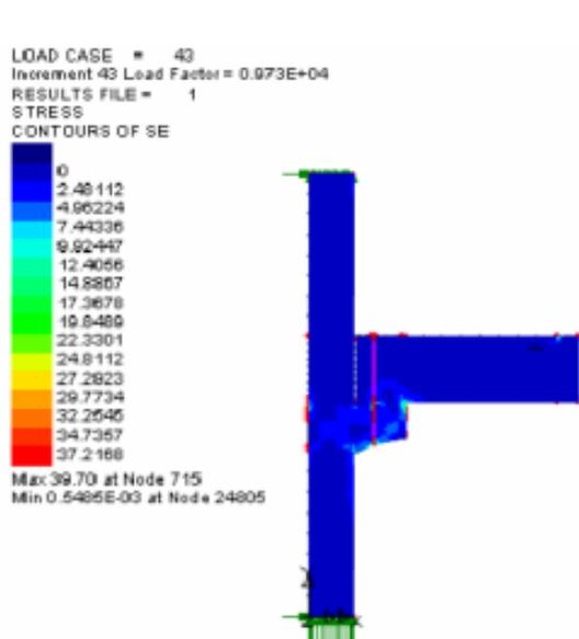
Figure 11: Von Mises Stress for Corbel Only Model
