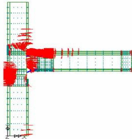
Figure 18: Crack Location for New Connection
