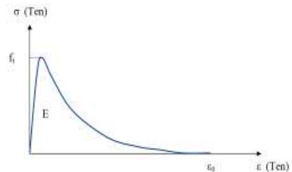
Figure 1: Tension Softening Behaviour of Concrete
