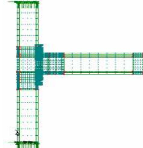
Figure 10: New Connection Plate 10mm and Bolt 22mm
