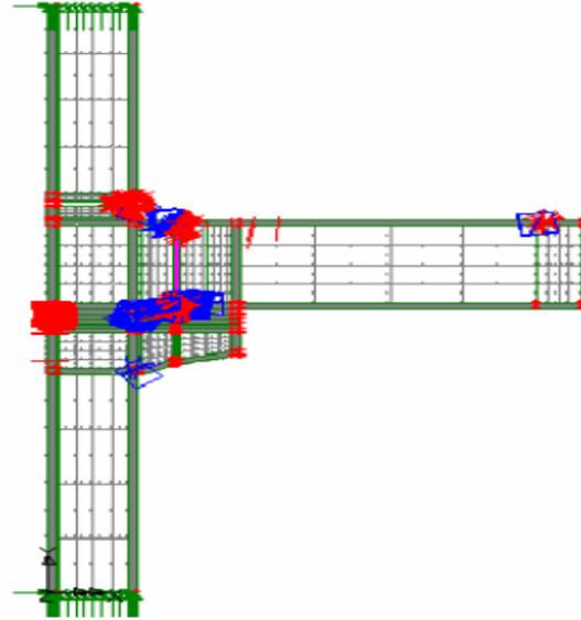
Figure 16: Crack Location for Corbel +Plate
