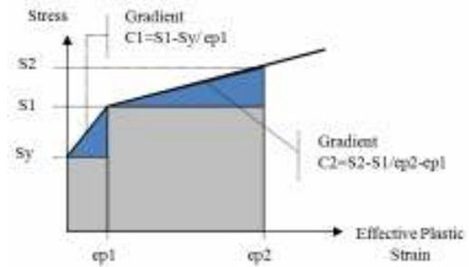
Figure 2: Hardening Properties of Steel
