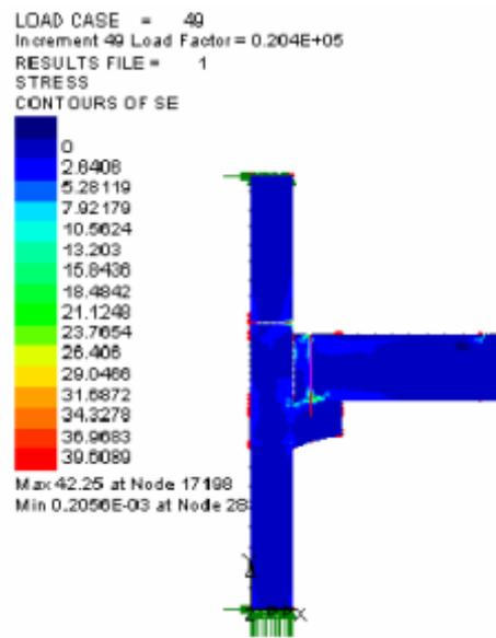
Figure 12: Von Mises Stress for Corbel +Plate Model
