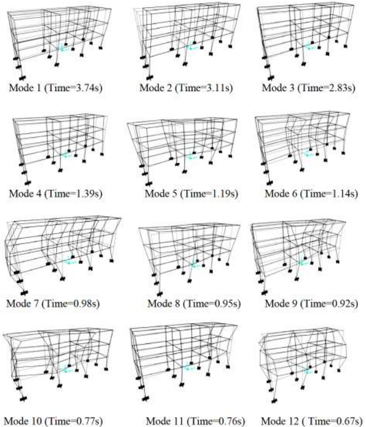
Figure 19: Deformed Mode for Modal Analysis (Proposed Connection)
