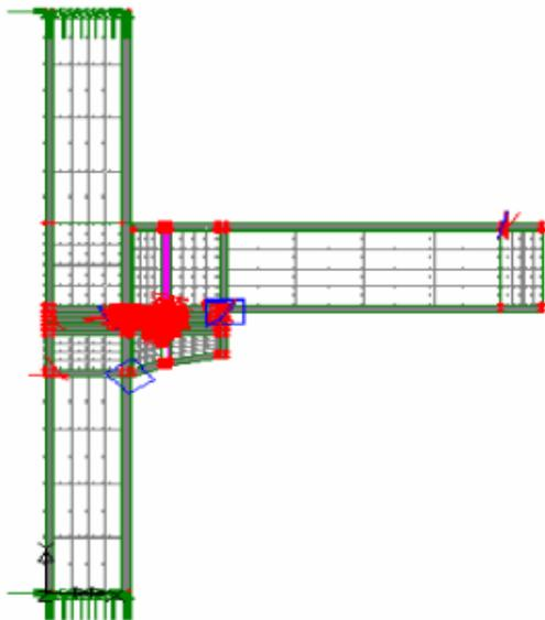
Figure 15: Crack Location for Corbel Only
