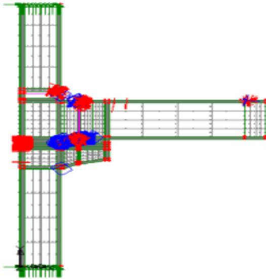
Figure 17: Crack Location for Corbel + Plate + Stiffener
