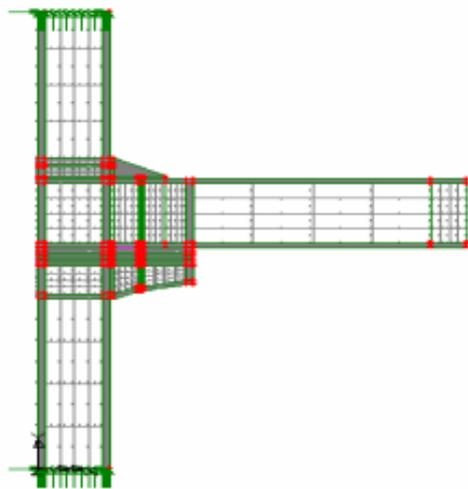
Figure 9: Corbel+ Plate and Bolt on Beam Top + Stiffener
