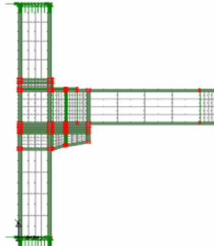
Figure 8: Corbel + Plate and Bolt on beam Top Model
