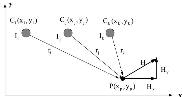
Fig.1. Magnetic field calculation for three conductor's lines
