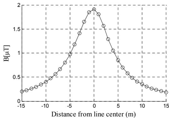
Fig.4. Magnetic field variation depending distance from line center at 3m height for 100A load current (34. 5kV MV-PDL).
