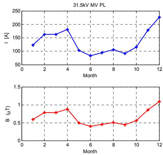
Fig. 7 Monthly based current load variation and magnetic flux for 31.5 kV MV-PDL.
