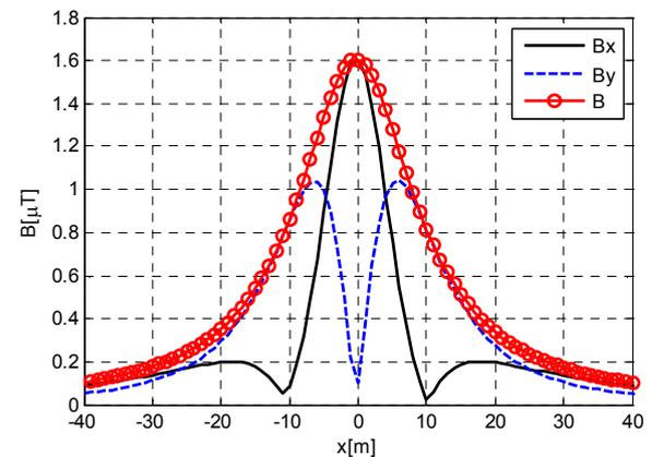
Fig. 5 MF variation at 1m height (31.5 kV MV-PDL with double circuits)
