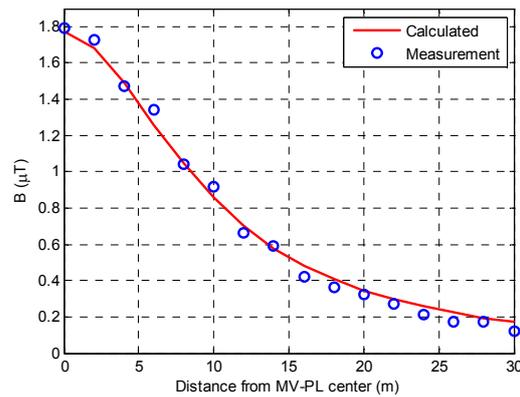
Fig. 8 Magnetic field variation from distance line center (at 1.5m height)
