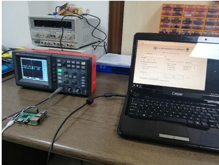
FIGURE 5. Sending the generated random numbers to Raspberry Pi wirelessly.
