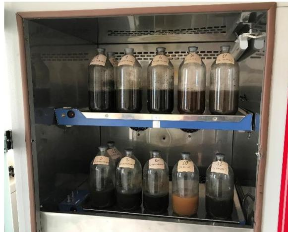
**Fig.1.** Experimental anaerobic batch study in shaking temperature control incubator
