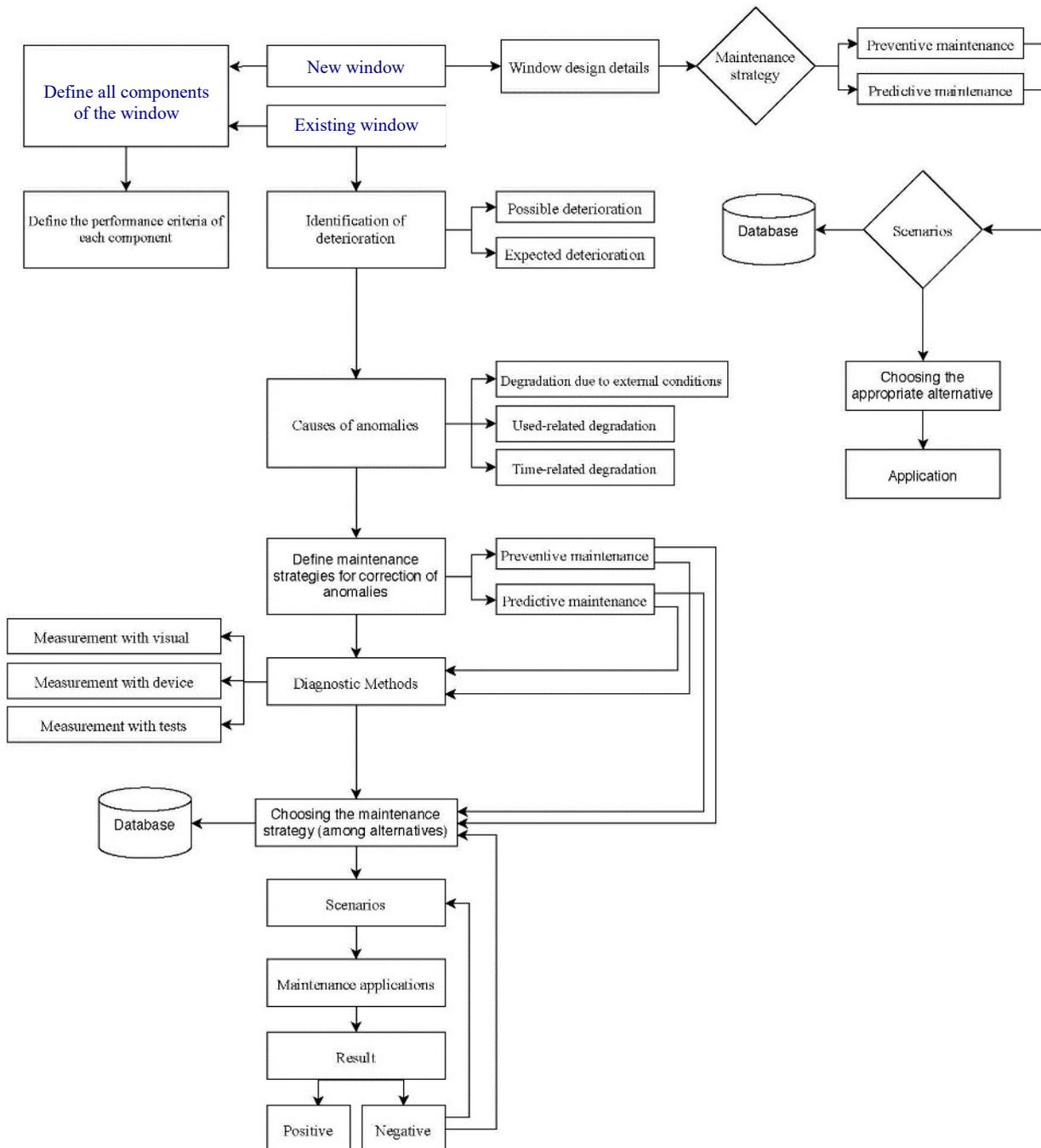
Figure 1 Workflow Chart for Window Maintenance Planning
