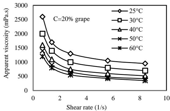
**Figure 3.** Variation of apparent viscosity with shear rates at different temperatures for a 20 % grape molasses in sesame paste
