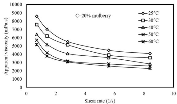
**Figure 2.** Variation of apparent viscosity with shear rates at different temperatures for a 20 % mulberry molasses in sesame paste
