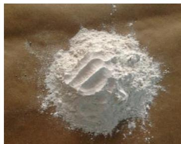
**Figure 4. Waste Marble Powder Sieved Through 0.25 mm Sieve**
