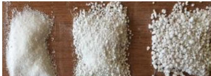
**Figure 1. Expanded Perlite Aggregates Sized as 0-2 and 2-4 mm**
