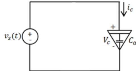
Figure 2. The CFD capacitor fed by a voltage source
