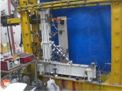
Figure 3 Cyclic steel beam-column connection tests, [14].
