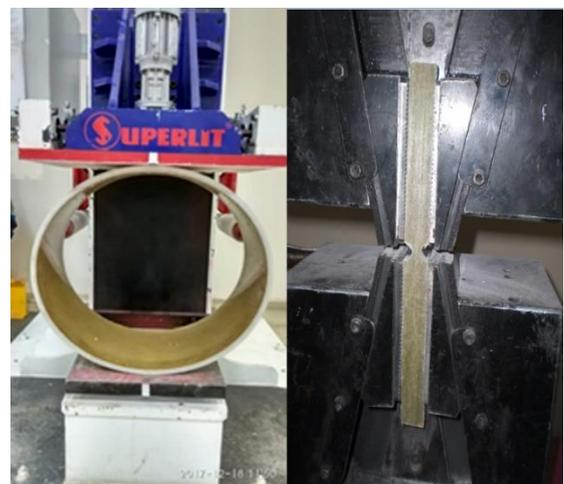
Figure 5 A visual of the specific ring stiffness and the LTS test
