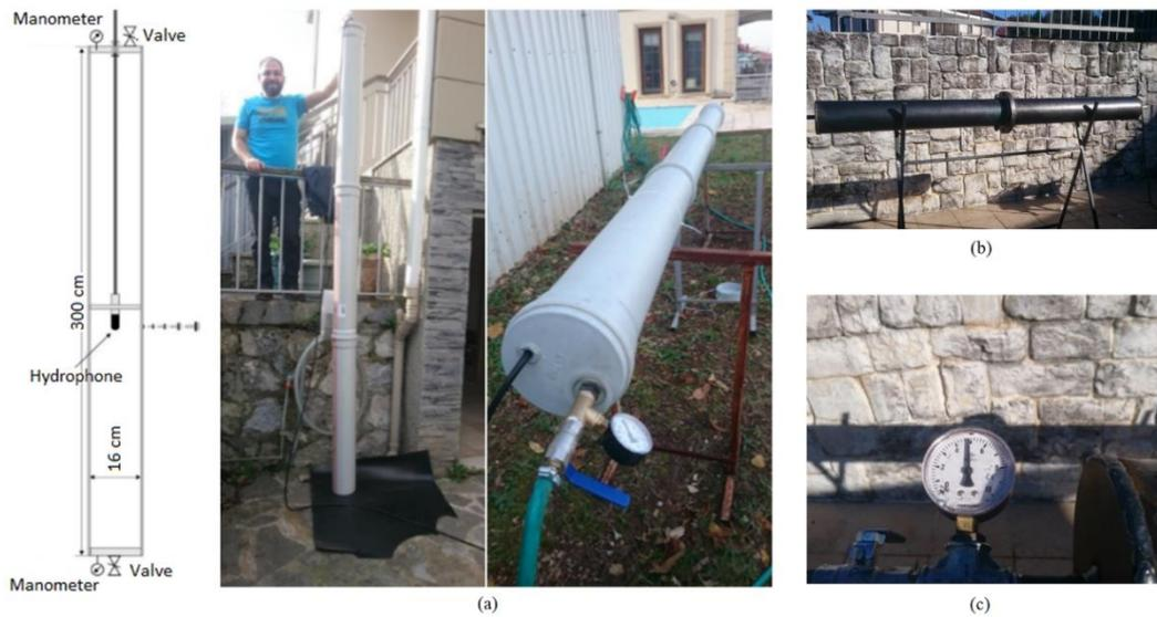
Figure 12 Sound mechanisms (a) PVC pipe assembly (b) Iron Cast pipe assembly (c) Manometer.
