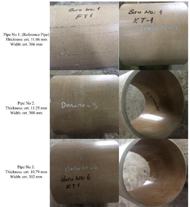
Figure 4 The stiffness test sample images of GRP pipes
