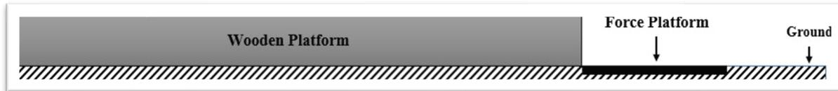
**Figure 1.** Instrumented staircase was used in this study. Height of wooden platform from ground = 0,15 m, length = 4 m. Force platform length = 0,6 m, width = 0,4 m.
