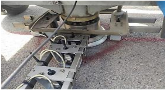
Figure 6. Placement of the falling weight deflectometer on the measurement point [12]
