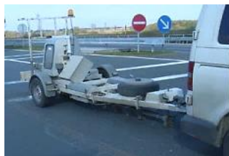
Figure 2. Falling weight deflectometer [22]
